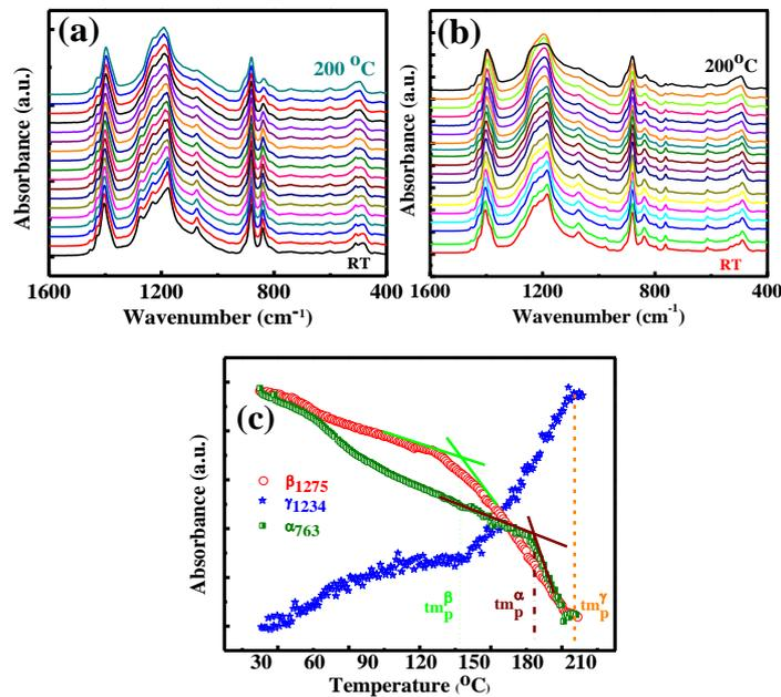
FIG. 3: In-situ thermal FT-IR spectra of (a) Ce-HFP and (b) HFP film with thermal ramp  $\sim 1$  °C/min, where the spectra in between room temperature 30 °C to 200 °C are shown in 10 °C interval for clarity. (c) The absorbance intensities of  $\beta$ -phase at 1275  $\text{cm}^{-1}$ ,  $\gamma$ -phase at 1234  $\text{cm}^{-1}$  from Ce-HFP film and  $\alpha$ -phase at 763  $\text{cm}^{-1}$  from HFP film for representing their peak melting temperatures via in-situ thermal FT-IR study.
