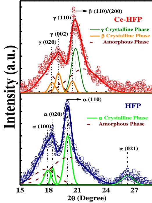
FIG. 1: XRD peak and its curve deconvolution from HFP and Ce<sup>3+</sup>-HFP films respectively, where the open circles are experimental data points and solid lines correspond to the best-fitted curves.
