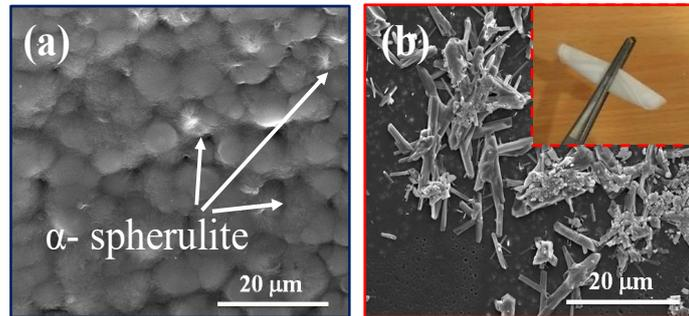
FIG. 4: FE-SEM images of the (a) HFP and (b) Ce-HFP films, inset of (b) represent the digital photograph of the composite film to demonstrate the flexibility.
