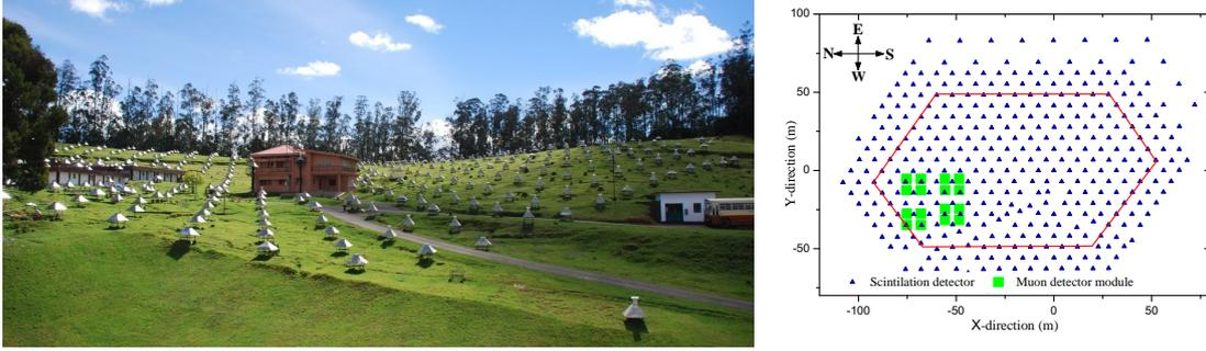
FIG. 1: The GRAPES-3 detector array with a varying elevation, showing muon detectors module in the left and data acquisition center in the middle of the figure. The figure on the right represents the schematic layout of the detector array.
