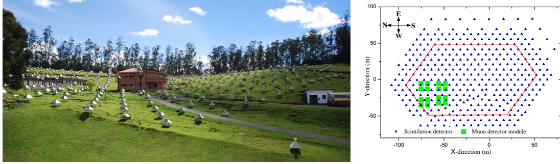
FIG. 1: The GRAPES-3 detector array with a varying elevation, showing muon detectors module in the left and data acquisition center in the middle of the figure. The figure on the right represents the schematic layout of the detector array.
